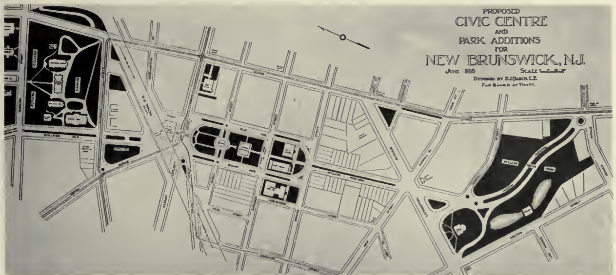
NEW BRUNSWICK.—A Comprehensive Scheme for the Rearrangement of a Portion of the Central District of the City, Involving the Clearance of Two City Blocks Near the Railroad Station, the Location of Civic Buildings Thereon, the Cutting-through of New Streets, and the Construction of a Parkway, etc.
