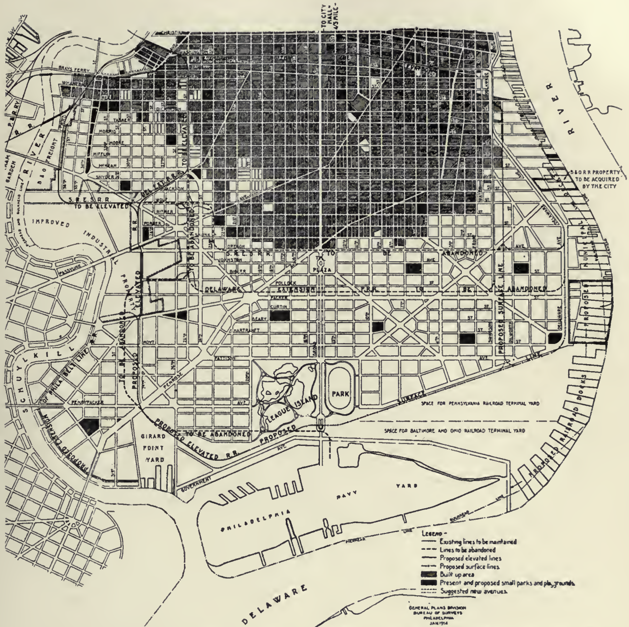
PHILADELPHIA.—Plan of South Philadelphia Improvement, Showing Main Avenues, Secondary and Minor Streets, Open Spaces at Important Intersections, Belt-Line Railroad, and Delaware Avenue Now Being Widened.
