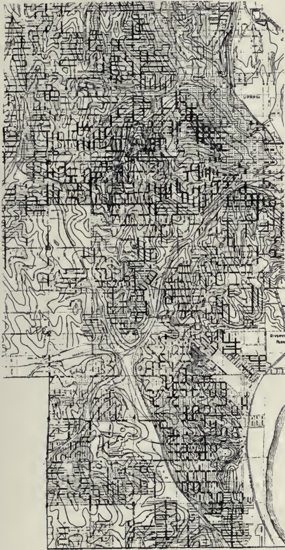
OMAHA.—Map Showing Contours and Gradients, Prepared by City Planning Commission. Grades from 5 Per Cent to 10 Per Cent Shown in Broken Lines; Grades of 10 Per Cent and More in Black.
