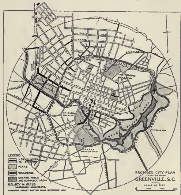
GREENVILLE.—Proposed City Plan, Showing Encircling Parks and Parkways and New or Widened Streets.
