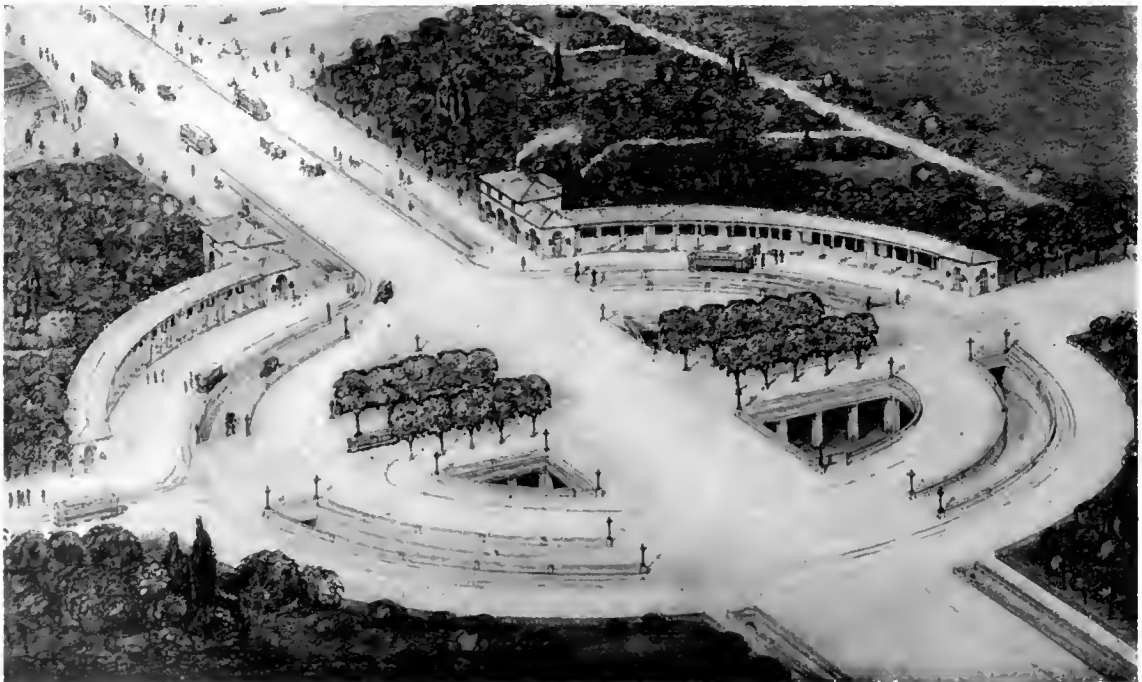
DETROIT.—Proposed Two-Level Traffic Separation Scheme at the Terminus of the Proposed Belle Isle Bridge.
