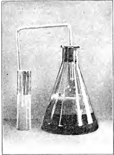
FIG. 95. Testing the gas from yeast fermentation with limewater
