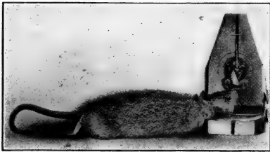
FIG. 89. The only rat this trap caught A poor design — wholly dependent on bait
