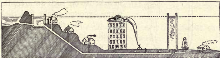
Distribution of water from a reservoir or a standpipe.
