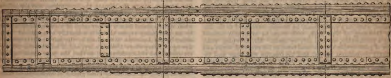
HALF SECTIONS, showing Bent Plates, Angle-iron Joint Covers, Stiffening Plates, &c.
