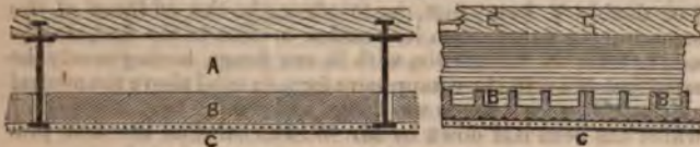
A. Hollow, or filled with Plaster. B. Tiles. C. Ceiling.
