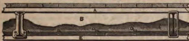
Cast-iron Chair. Wrought-iron Chair. A. Joist. B. Hollow. C. Plaster. D. Square iron. E. Flat iron tie.
