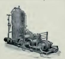
Hoisting Engine With Boom Swinger
