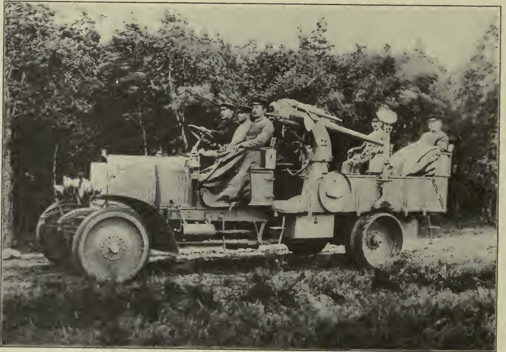
AUTOMOBILE GUN, ESPECIALLY DESIGNED FOR ATTACKING AIRCRAFT Motor Tractors and Guns Mounted on Automobiles Were an Outstanding Feature of the Swift German Advance Through Belgium and France
