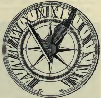
FIG. 54.—Style and dial of a horizontal sundial.
