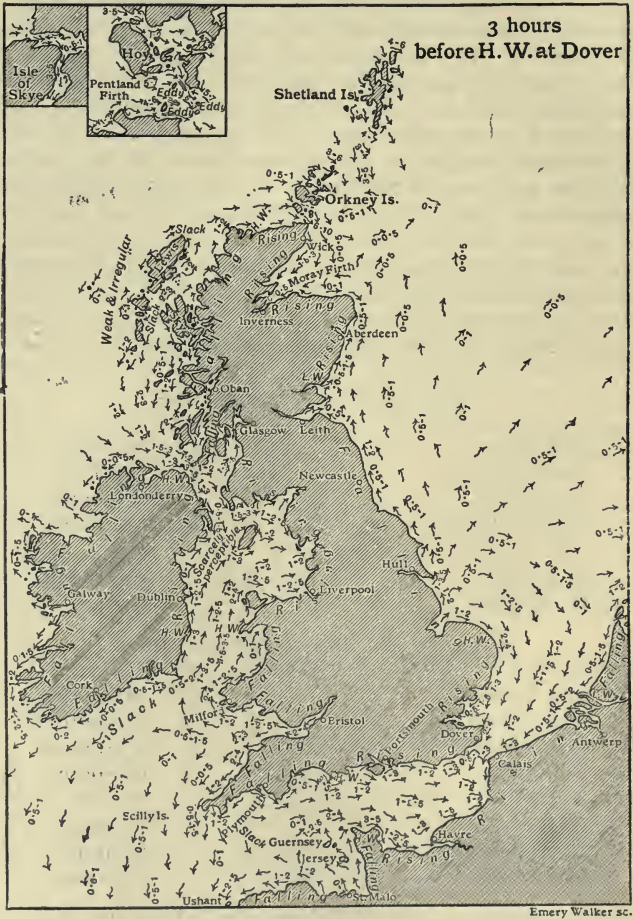
FIG. 155.—Chart of tidal streams 3 hours before high water at Dover. (Speeds are given in knots, that is, nautical miles per hour.)
