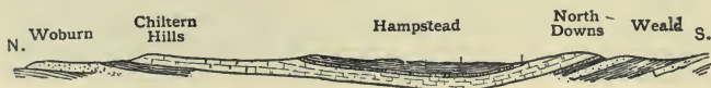
FIG. 147.—Geological section from Woburn through London to the North Downs, showing the syncline of the London Basin.
