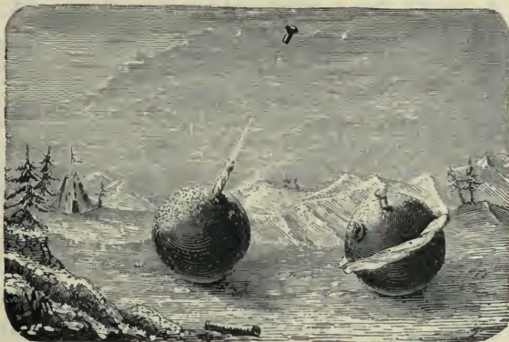
FIG. 180.—To illustrate the force of expansion of freezing water.
