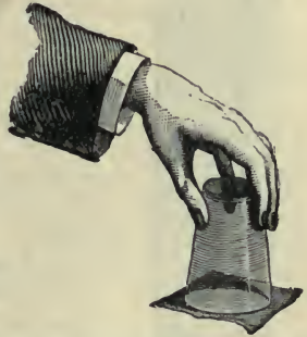
FIG. 190.—Experiment illustrating the pressure of the atmosphere.
