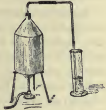
FIG. 141.—Experiment to show that tap water contains dissolved carbon dioxide.
