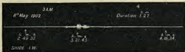
FIG. 115.—Long-distance seismogram of the eruption of Mont Pelée (p. 173) on May 8, 1902, obtained by Prof. J. Milne in the Isle of Wight.
