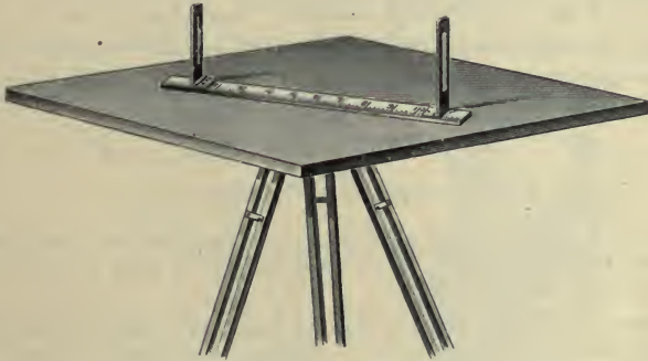
FIG. 8.—Sight-rule on plane table.
