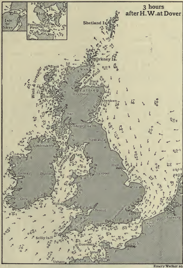
FIG. 156.—Chart of tidal streams 3 hours after high water at Dover. (Speeds are given in knots, that is, nautical miles per hour.)
