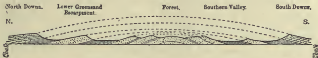
FIG. 148.—General geological section of the Weald and its relation to the North and South Downs. The dotted lines indicate the original strata which have been removed by denudation. (Adapted from the Proceedings of the Geologists' Association , 1897.)
