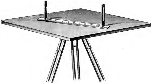
FIG. 8—Sight-rule on plane table.
