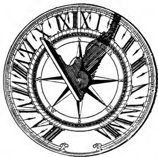
FIG. 54.—Style and dial of a horizontal sundial.
