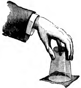
FIG. 190.—Experiment illustrating the pressure of the atmosphere.
