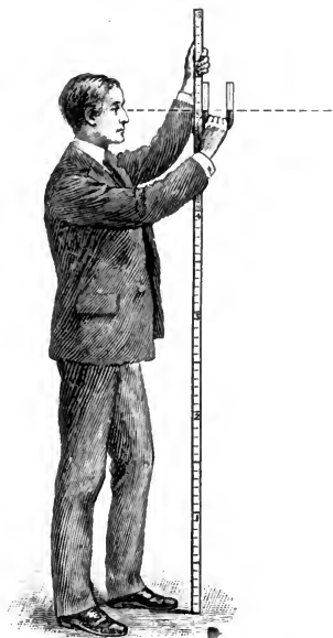
FIG. 9.—A simple water-level and levelling staff used for measuring relative heights.
