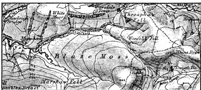
FIG. 12.—A hachured and contoured map. A portion of Sheet 59 of the Ordnance Survey one-inch map. Scale 1" = 1 mile. (Compare with Fig. 15.)
