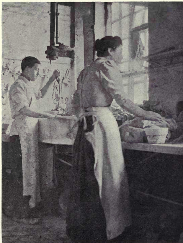
FIG. 24 MAKING CUPS ON JIGGER
