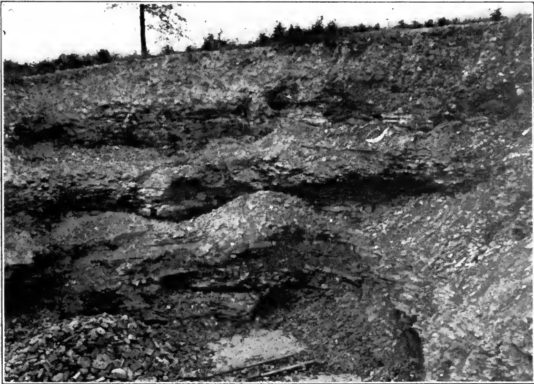
FIG. 2.—Bank of (Devonian) shale used for paving-brick, Cumberland, Md. (After H. Ries, Md. Geol. Surv., IV, p. 454, 1902.)
