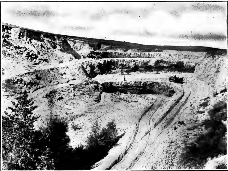
FIG. 2.—Tertiary clays (Ione formation) used for brick, terra-cotta, etc., Lincoln, Calif. (Photo loaned by Gladding, McBean & Co.)
