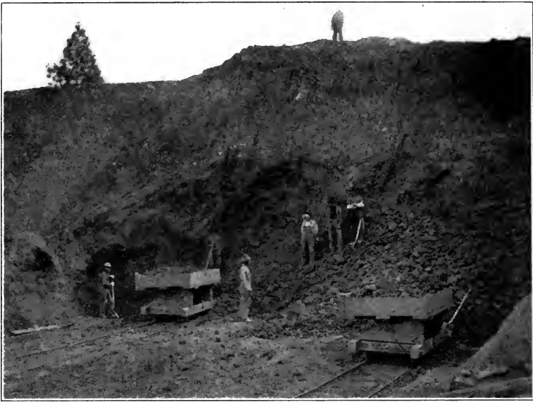
FIG. 1.—Red-burning brick-clay bank at Freeman, Wash. (Photo loaned by Washington Brick, Lime, and Mfg Co.)
