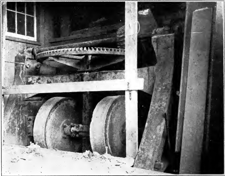
FIG. 1.—Dry pan used for grinding hard clays, shale, and brick. (After H. Ries, N. Y. State Museum, Bull. 35, p. 765, 1900.)
