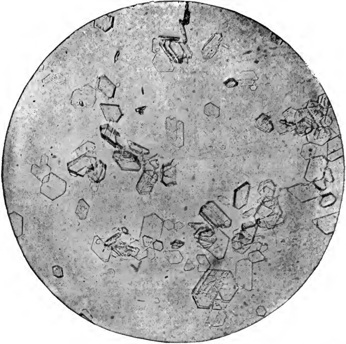
FIG. 1.—Photo-micrograph of kaolinite. (After Merrill, Non-metallic Minerals .)
