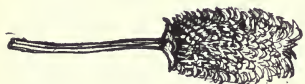
FIG. 126. — This is the teasel which is used to brush the nap of the cloth in finishing. These small thistles are arranged in rows in the machine rollers through which the cloth passes.
