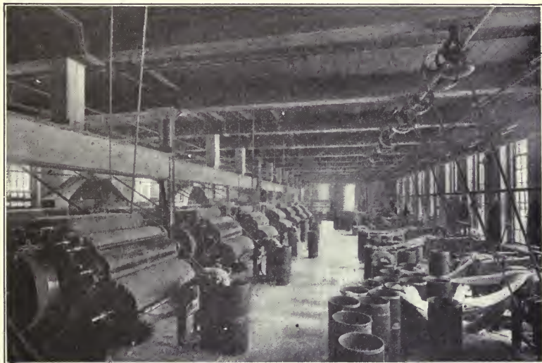
FIG. 122. — Wool carding. Notice the round cylinders. The gauzy web is being delivered into the can in front of the carding machine.
