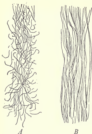
FIG. 124. — This shows the difference in the slivers of wool and worsted yarn. A is the woolen yarn, well mixed; B is the worsted yarn, well combed.
