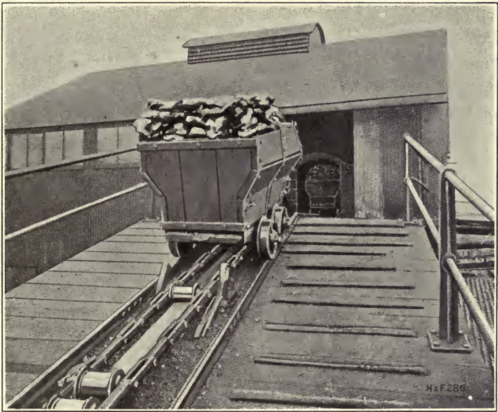
FIG. 28.—Creepers, for elevating tubs by mechanical means. Reproduced by kind permission of Messrs. Heenan and Froude, Birmingham.
