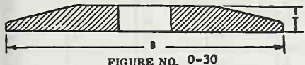
FIGURE NO. O-30 Driving flange secured to spindle for use only on portable wheels with threaded inserts or projecting studs.
