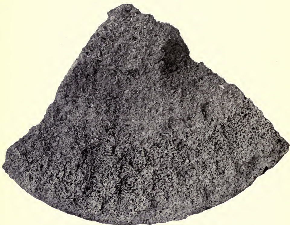
FIG. 8. B-21. COKE FROM EQUAL PARTS OF VERMILION COUNTY COAL AND COKE DUST
