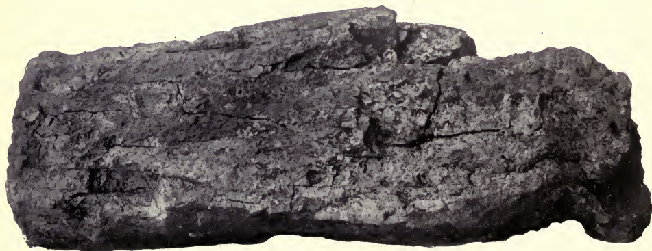
FIG 13. B-30. 48-HOUR COMPRESSED SOLVAY COKE
