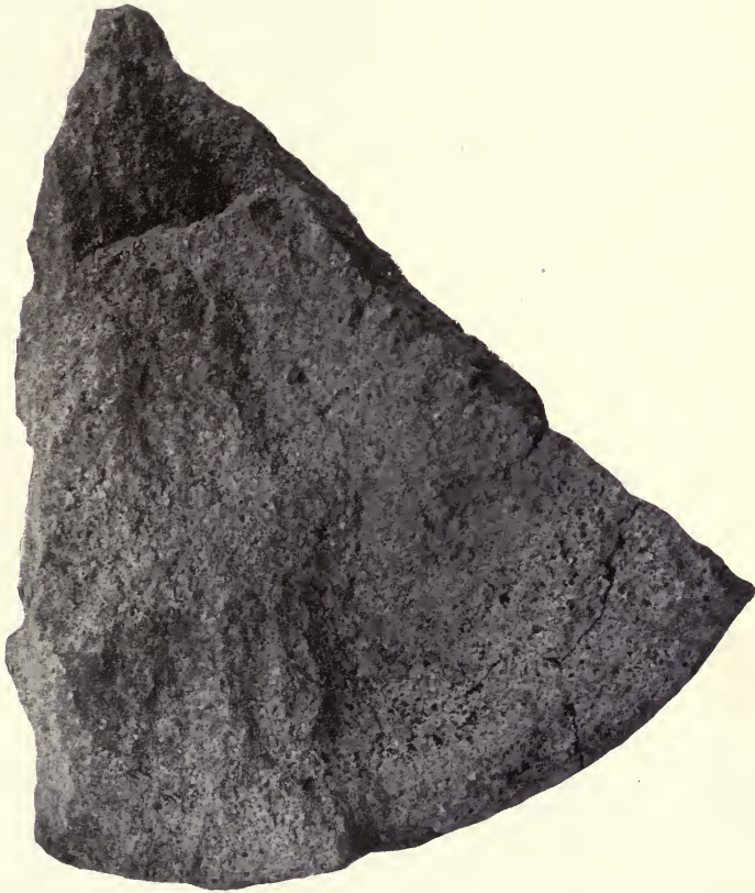
FIG. 11. B-13. COKE FROM SALINE COUNTY COAL AND COKE DUST
