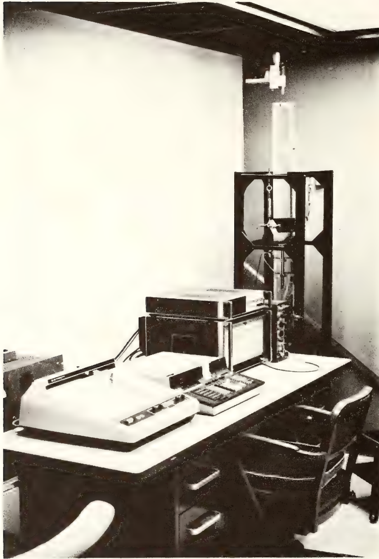
Fig. 1. View of the total ARSA system showing fall tube and associated electronics.
