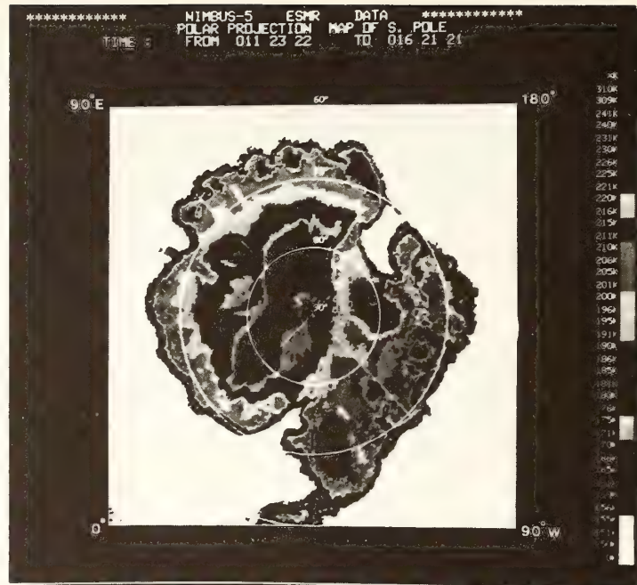
Fig. 7. Microwave image of the Antarctic continent with brightness scales affixed made from the ESMR on Nimbus 5 during January 1973 (NASA Goddard Space Flight Center).
