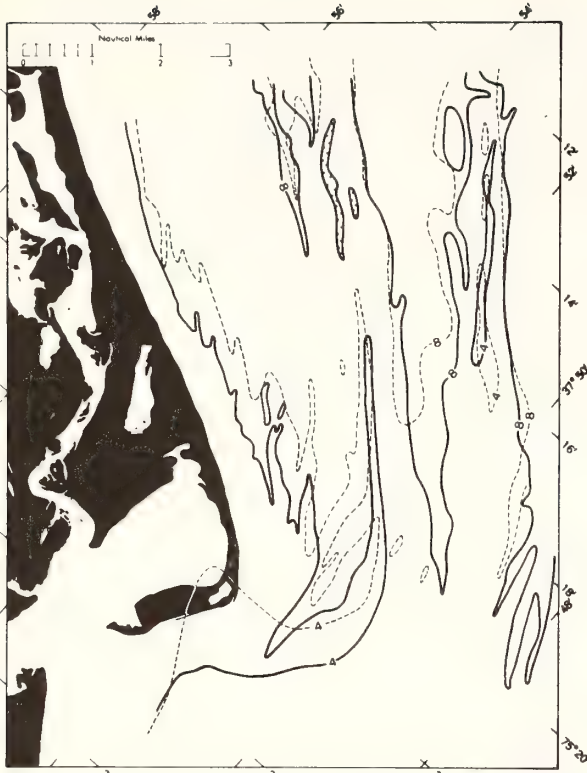
FIGURE 36. Bathymetric time series of Chincoteague shoals, Delmarva (Delaware-Maryland-Virginia) coastal compartment. Ridges have migrated slightly offshore, and have extended their crestlines markedly to the south between the Coast and Geodetic surveys of 1881 (dashed line) and 1934 (solid line). From Duane et al. (1972).
