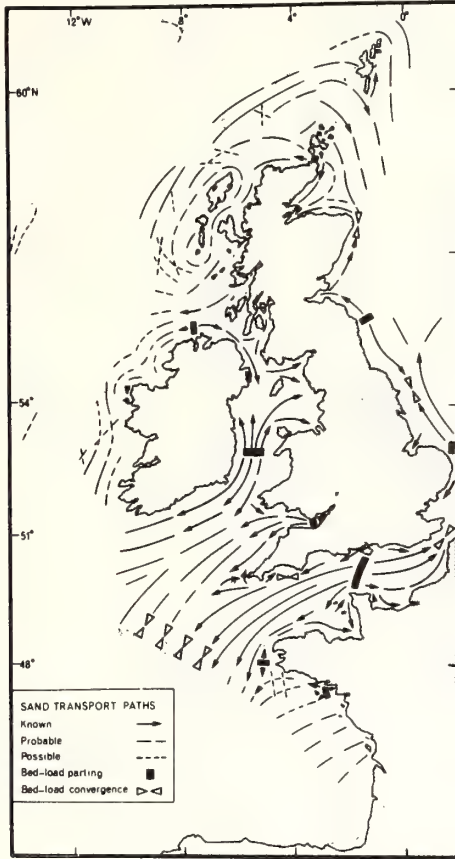
FIGURE 26. Generalized sand transport paths around the British Isles and France, based on the velocity asymmetry of the tidal ellipse and the orientation and asymmetry of bed forms. From Kenyon and Stride (1970).
