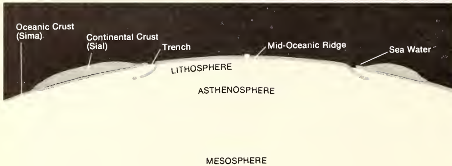
The shells forming the earth are dynamic. Convective circulation high in the mantle (asthenosphere zone) transports the topmost region of the mantle as well as the crust. The landmasses are buoyed along on the spreading lithosphere. (After Isacks, Oliver, and Sykes [1968].)
