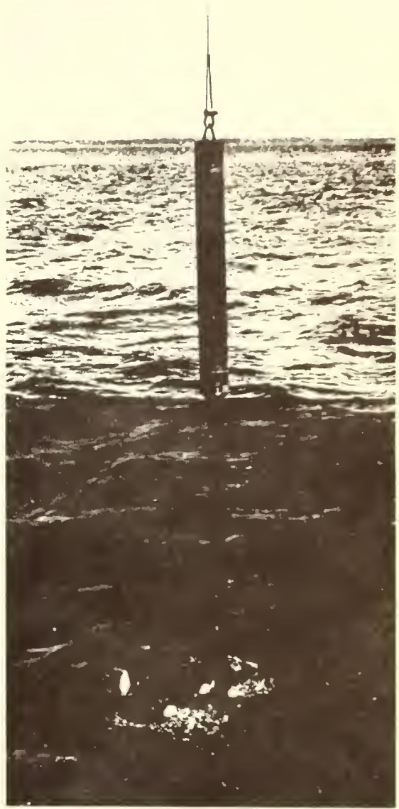
Fig. 2 Bottom-sediment density single-barrel probe.
