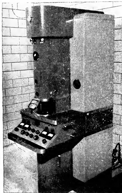
FIGURE 5. Electron microscope. It uses a beam of electrons and magnetic fields, which take the place of light and lenses. Magnifications of over 100,000 times (diameters) may be obtained. This microscope is useful in studying the smallest living things such as viruses and the submicroscopic structures of cells. (Photo courtesy of George Jennings, Michigan Department of Health.)
