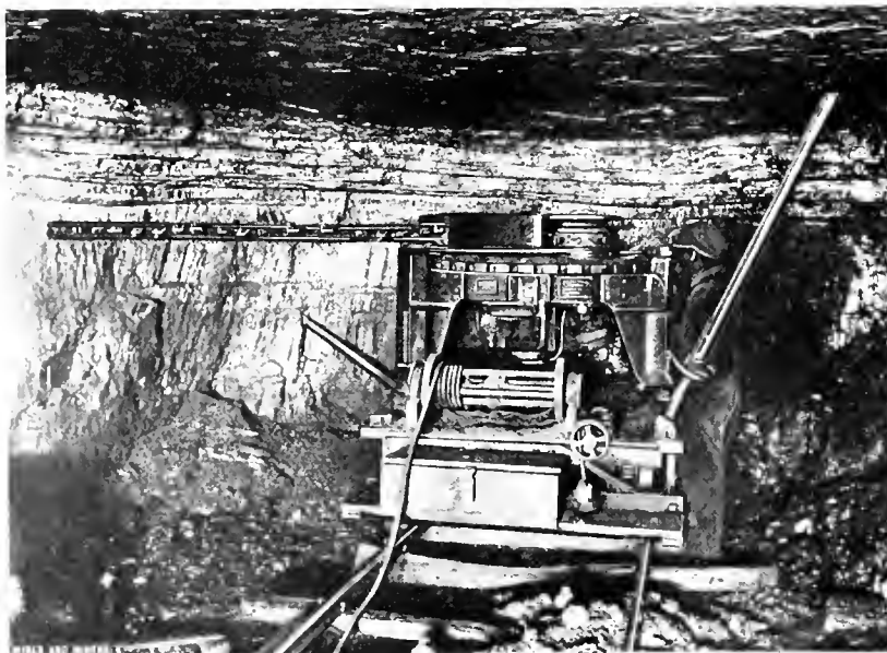
FIG. 1. JEFFREY-O'TOOLE COAL CUTTER
