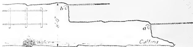
FIG. 2. PLAN OF ENTRY READY FOR BLASTING
