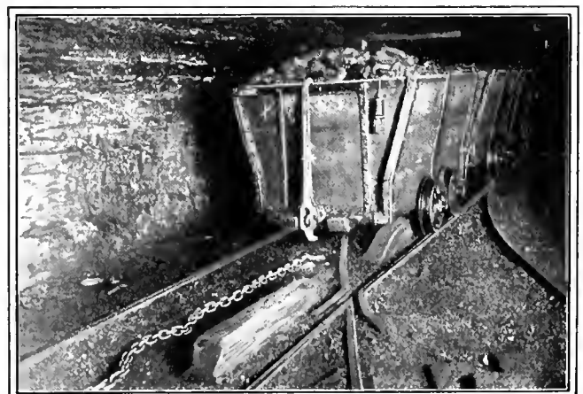
FIG. 5. NEW ARRANGEMENT FOR RELEASING TAIL-ROPE
