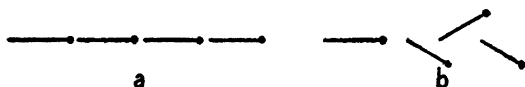
FIG. 87.—Association colloids. a , associated soap molecules at low temperature; b , disrupted dipole chain at high temperature.
