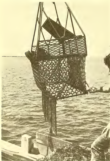
Fig. 8 - Oyster dredge with teeth angled forwards, to pass under oysters laying on bottom. Hinged door at bottom of dredge unlatches to release load of oysters.
