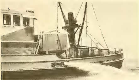
Fig. 10 - Spreading quicklime to kill starfish which invaded oyster bed. Tank on boat holds 15 tons of quicklime.
