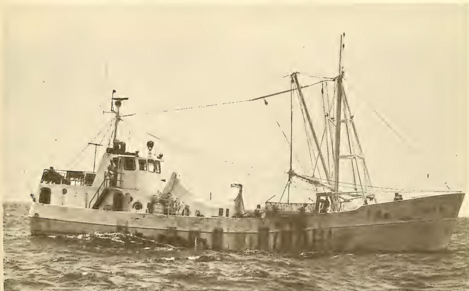
Fig. 2 - Factory scalloper Ruth M., 86-foot steel hull, fully automated to process calico scallops at sea, operating on Cape Kennedy grounds.
