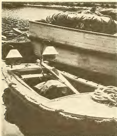
Fig. 6 - A skiff outfitted with lights for attracting pelagic fishes. In 1968 about 4,000 of these units engaged in the Yugoslavia fishery for sardines, sprat, and anchovies, and the other open-water species.
