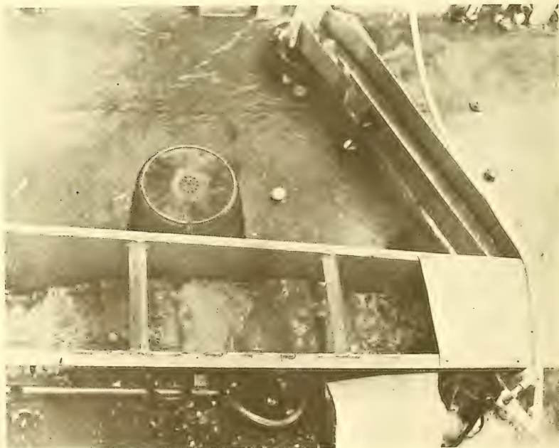
Fig. 11 - Salt-water floatation cleaning trough and conveyor trough leading to below-deck eviscerator.
