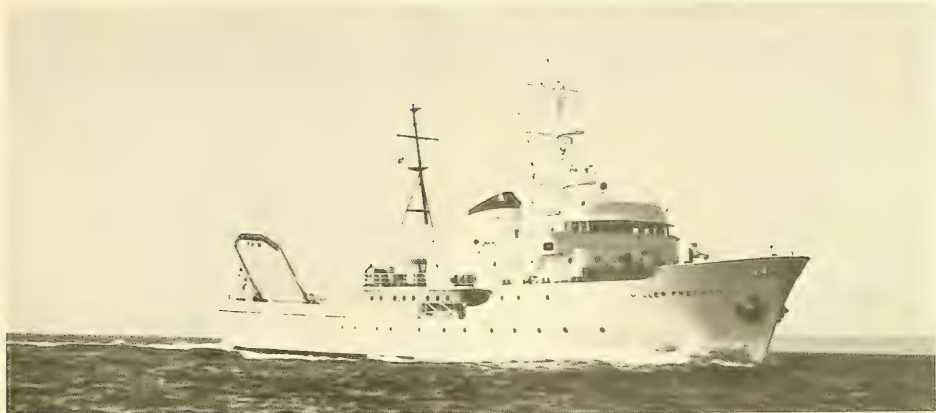
Fig. 3 - The bathysphere can be lowered and raised with the trawling winches, cables, and gantry that are permanently installed aboard the 215-foot Miller Freeman, the Seattle Biological Laboratory's research vessel.
