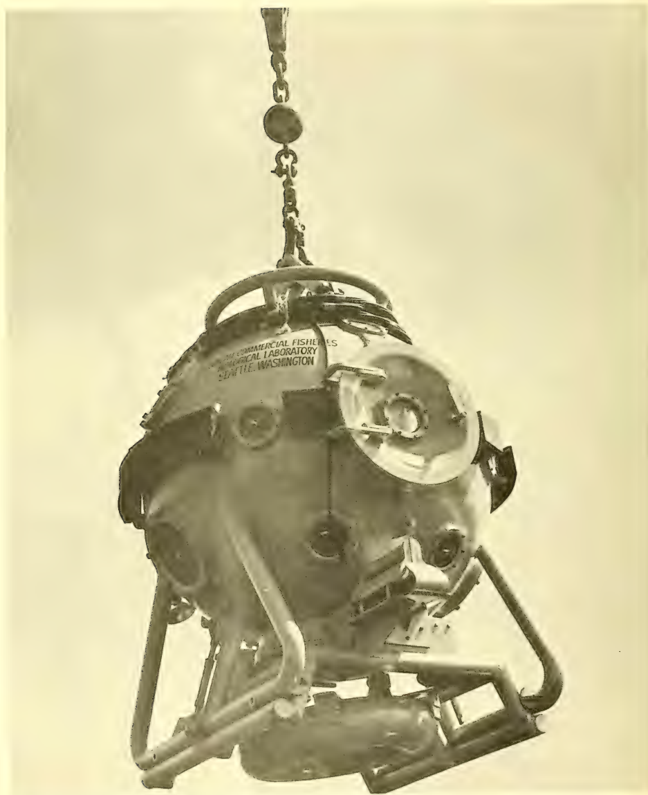
Fig. 1 - BCF's new bathysphere will transport two observers at atmospheric pressure to a depth of 675 feet. The bathysphere is about 8 feet high and weighs nearly 9,300 pounds (including 2,500 pounds of ballast).
