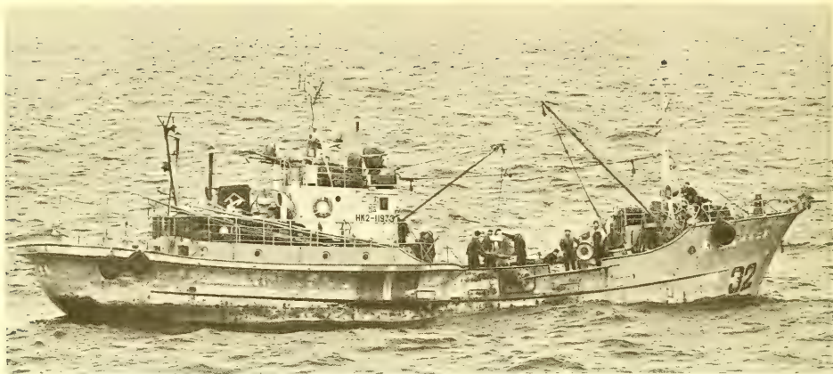
Fig. 6 - A Japanese ship, about 90 feet long, retrieves tanner crab pots. Groundline comes aboard over power roller at starboard rail. (Photos: M. C. Zahn)
