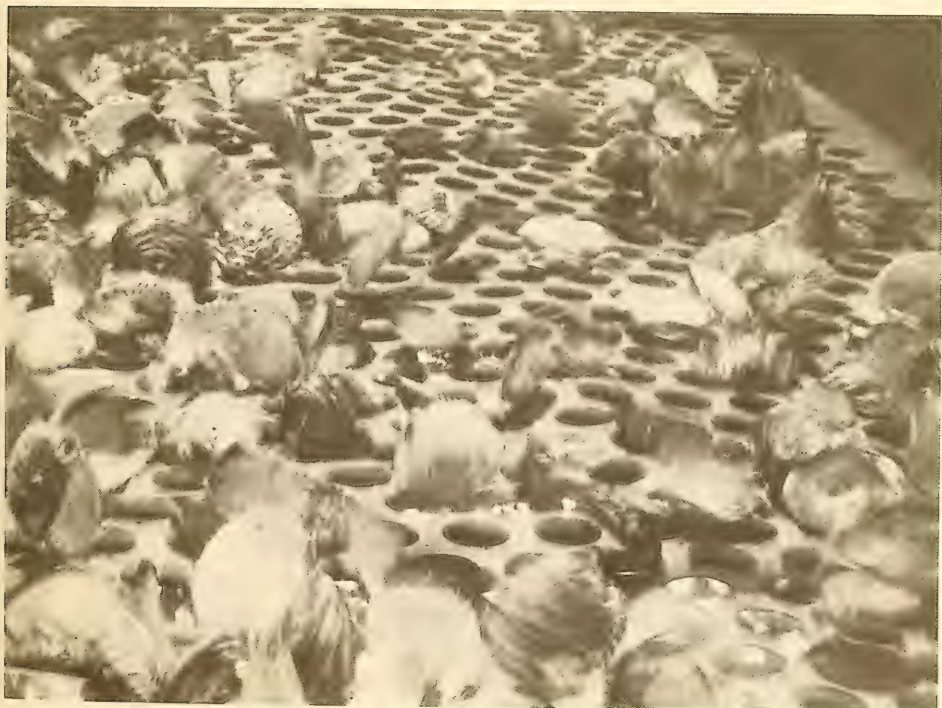
Fig. 9 - Vibrating shaker screen separating shells from shucked scallop meats. The meats drop through perforations in the screen.
