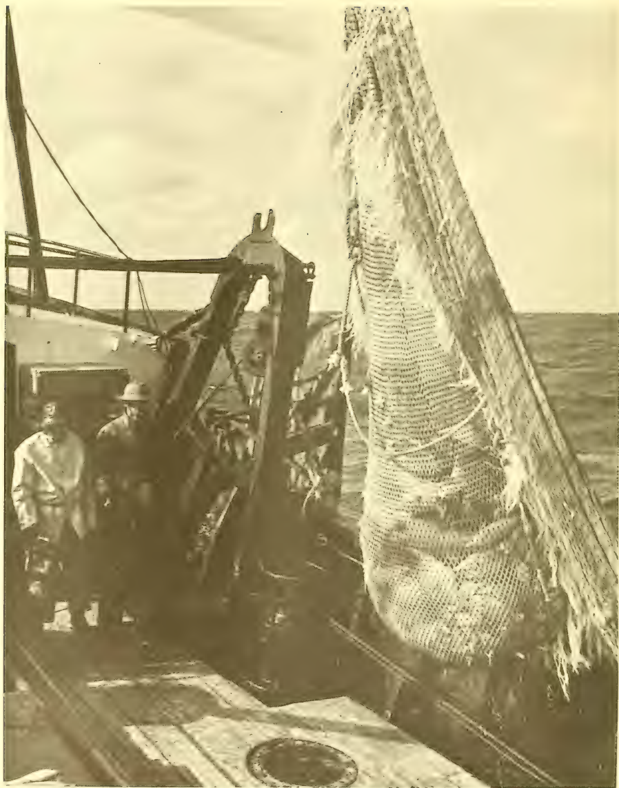
Cod-end swinging aboard BCF-chartered vessel during explorations off South Carolina. (Photo: J. B. Rivers)
