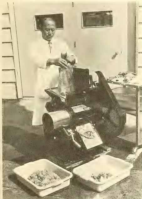
Fig. 1 - This Japanese machine separates fish flesh from skin and bones. It was put to use recently by scientists at the BCF Fisheries Technology Laboratory in Seattle, Washington. The machine was used during cooperative U.S.-Japan studies on increased use of latent Northeast Pacific fishery resources. BCF scientists believe the potential for mechanizing the process of flesh separation and recovery could lead to a new concept in fish utilization and processing in the U.S.
