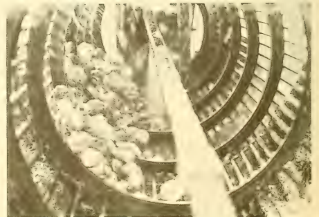
Fig. 6 - Inside view of rotating screw-type squirrel cage "separator."
