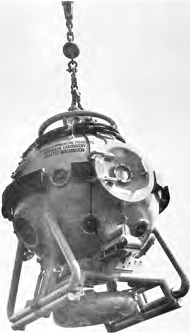
Fig. 1 - BCF's new bathysphere will transport two observers at atmospheric pressure to a depth of 675 feet. The bathysphere is about 8 feet high and weighs nearly 9,300 pounds (including 2,500 pounds of ballast).
