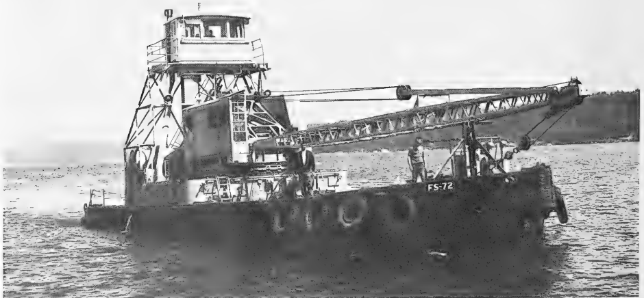
Fig. 2 - The bathysphere's self-propelled support barge, a converted airplane salvage barge, 104 feet long, has a cruising speed of about 8 knots; it carries two scientists and a crew of three. The crane on the barge is capable of lifting 15 tons.
