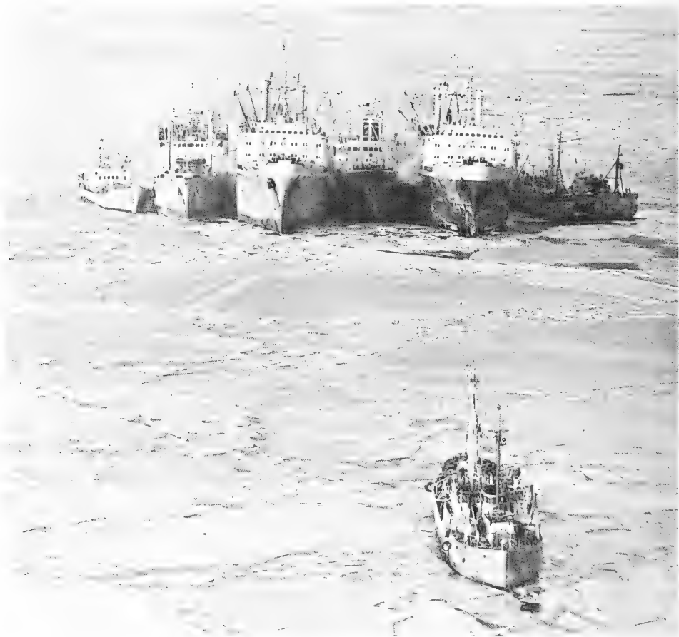
Fig. 4 - Far removed from stormy seas, 7 Soviet vessels--from motherships to medium side trawlers--nest together to transfer fish and cargo while another side trawler approaches to make delivery. The vessels belong to the Soviet herring fleet operating near St. Matthew Island in the Bering Sea, and are anchored some 30 miles, or more, from the ice, but it is common practice for the ships to take shelter from seas and icing conditions by running inside the ice. All Soviet vessels in this winter fishery are reinforced for travel in pack ice. (Photo: M. C. Zahn; Date: December 31, 1969.)
