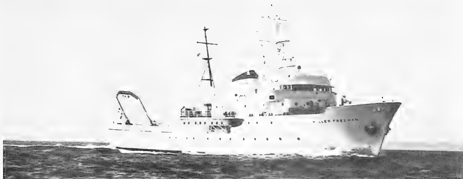
Fig. 3 - The bathysphere can be lowered and raised with the trawling winches, cables, and gantry that are permanently installed aboard the 215-foot Miller Freeman, the Seattle Biological Laboratory's research vessel.
