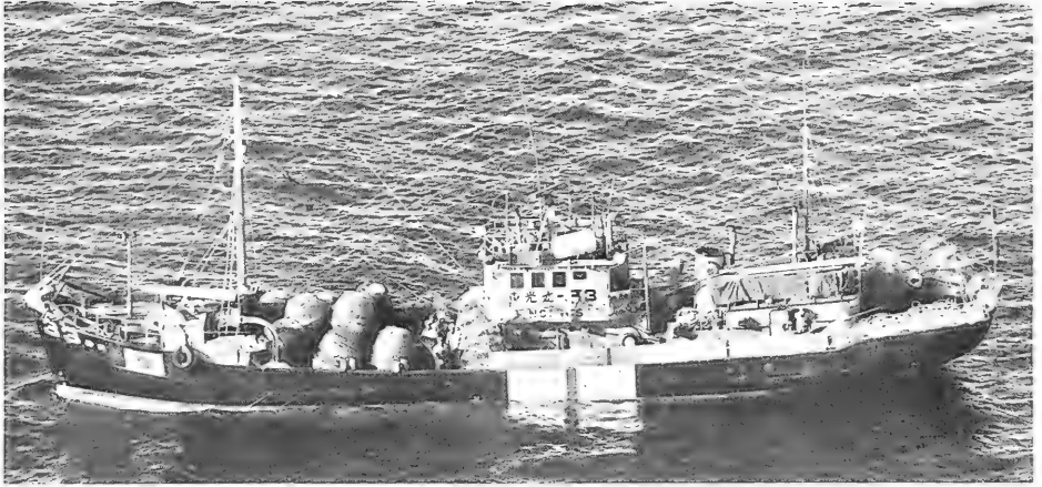
Fig. 2 - A tanner crab pot vessel, assigned to mothership 'Keiko Maru,' sets gear north of Unimak Island. A buoy and flag are visible going over stern. Stacks of nested pots are on well deck, and fully assembled pots are on fantail.
