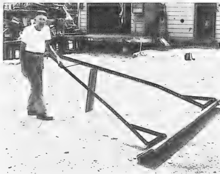
Fig. 2 - Cutting board, or vane, is towed rapidly over bottom, at angle shown, to scour silt off shells. Currents carry suspended silt off bed.
