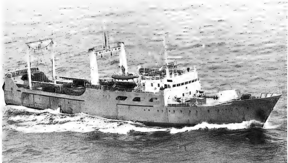
Fig. 5 - The South Korean stern trawler 'Kang Wha 601' is one of two similar ships which have operated off Alaska since 1968. Built in France in 1966, she is 252 feet long, 1,518 gross tons, with accommodations for a crew of 48. Equipped to both catch and process fish, she has a 900 cu. m. hold capacity and an 18 ton a day sharp freeze capability.
