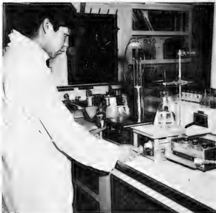
Fig. 2 - Trainee measures dissolved oxygen in floating laboratory's water supply. The training emphasizes learning to measure--and to understand importance of--the properties of water that are vital to the mariculturist.
