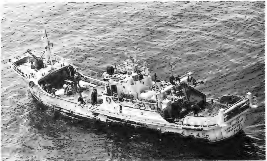
Fig. 2 - The 'Kook Yang No. 118' retrieving a gillnet. Five of these gillnetters operated in the 1969 high seas salmon fisheries off Alaska. They are 107 feet long, 133 gross tons, and appear to be the same basic ship as the seven Kook Yang otter trawlers operating in the same area.
