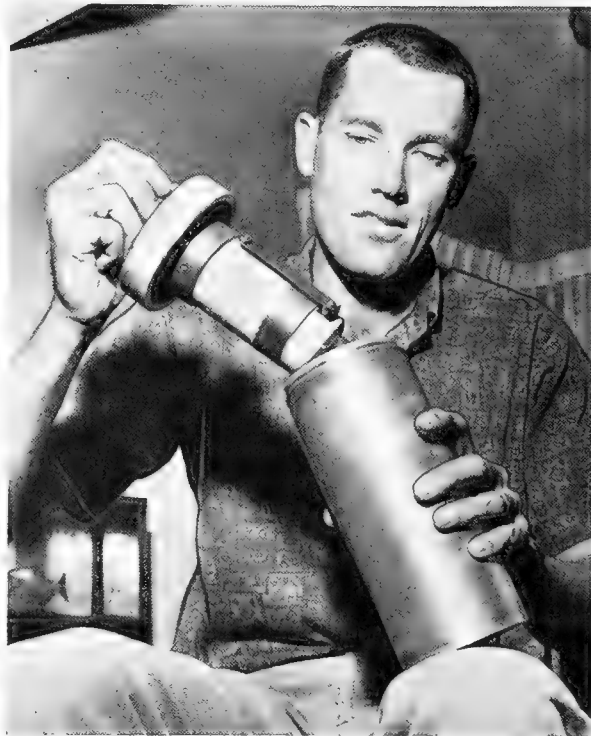
Frank J. Hester, the inventor, holds bathykymograph which can tell how fast and deep a fish net sinks.
