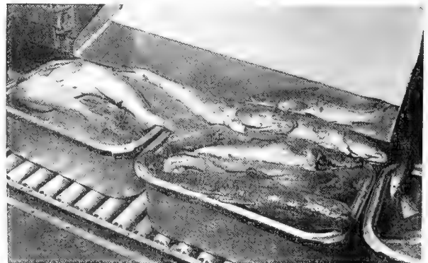
Fig. 4 - After four hours of treatment by carefully regulated temperature, humidity, and high-velocity air, the fish blocks emerge from the thawing unit as individual fish ready for filleting.
