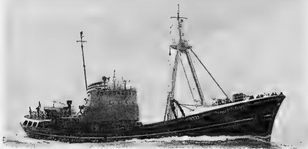
Silver Cod Trophy winner in 1963. The Stella Leonis is fitted for starboard fishing only. Accommodations are provided amidships and aft for 30 persons. The fish-storage hold has a capacity of 18,170 cubic feet. The vessel is powered by a 1,800-horsepower Diesel engine.
