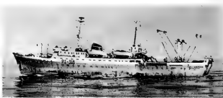
Fig. 5 - Stern trawler of the Maiakovskii class. Known also as a BMRT , the vessel is a completely integrated fishing and processing factoryship with freezing, canning, and reduction equipment.
