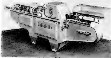
Fig. 1 - A new fish-gutting and beheading machine marketed by a West German manufacturer.
