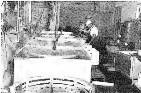
Fig. 36 - Open tanks can be used, since pasteurization temperatures are below boiling. Tanks in background are used to cool the cans of pasteurized meat.
