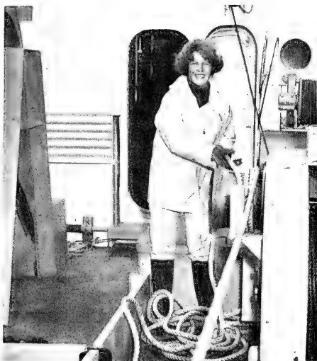
Fig. 2 - Young girl hauls in bull rope at deck capstan on Canyon Prince , in a demonstration of automated net-handling equipment requiring a single deckhand.
