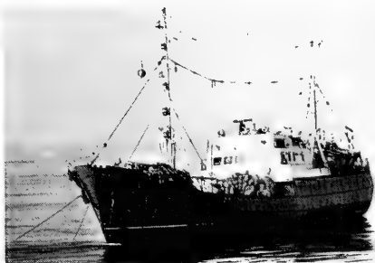
Fig. 4 - Trawler of Okean class. Has refrigerated holds. Vessel uses conventional side trawl, and is also equipped for gill-netting.
