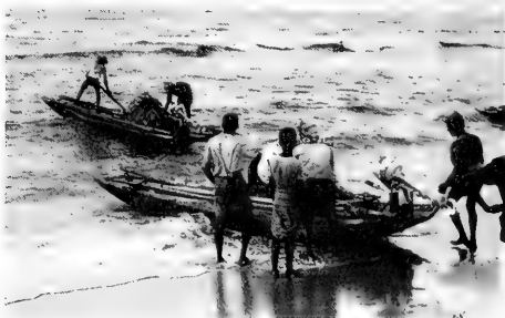
Ceylonese fishermen launch their shallow log raft teppans. Tests have proved that these craft, which can slide over coral and sand reefs and budge ashore on any beach, can catch more fish if mechanized with outboard engines.
