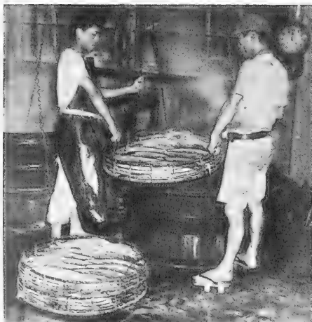
FIGURE 6 - PLACING A BASKET OF SKIPJACK FILLETS INTO A COOKING VAT FOR STEAMING. "THESE ARE THEN SMOKED AND DRIED FOR MAKING 'KATSUOBUSHI.'"
