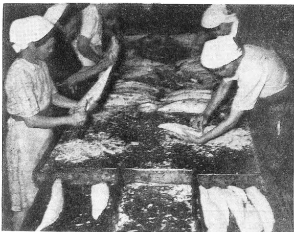
FIGURE 3 - THE DARK MEAT AND BLOOD SPOTS ARE REMOVED FROM THE ALBACORE TUNA LOINS.
