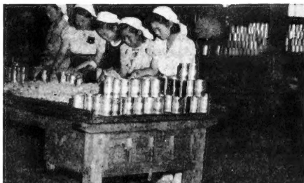
FIGURE 5 - PACKING DISCARDED SCRAPS OF ALBACORE WITH SOYA SAUCE IN TALL CANS FOR CONSUMPTION IN JAPAN.
