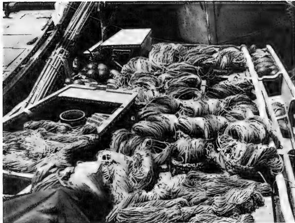
FIGURE 9 - DRYING LONG LINES IN PORT. HERE THE COILED SECTIONS OF EACH BASKET HAVE SIMPLY BEEN SEPARATED AND ALLOWED TO REMAIN IN THE BASKET.
