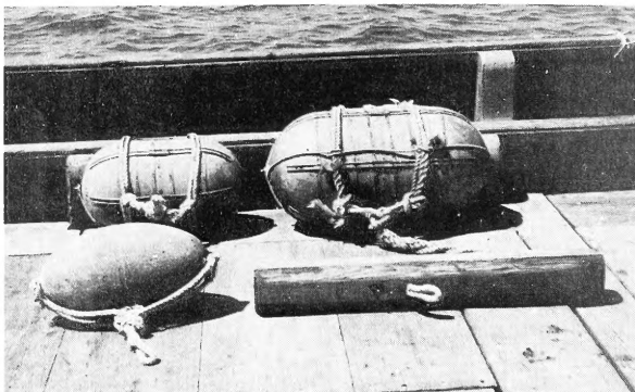
FIGURE 6 - FLOATS USED IN THE HAWAIIAN LONG-LINE FISHERY. THE ALUMINUM OXYGEN TANKS AND THE GALVANIZED METAL FLOATS ARE USED TO SUPPORT THE MAIN LINE AT THE CENTER OF A BASKET. THE WOODEN FLAGPOLE IS FASTENED TO THE FLAGPOLE AND IS ATTACHED AT THE "HEAD" OF THE BASKET.
