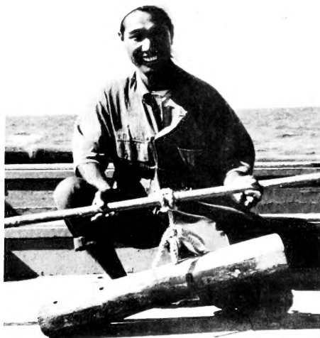
FIGURE 7 - ATTACHMENT OF WOODEN FLOAT TO THE FLAGPOLE. NOTE THAT THE LOOP ON THE FLOAT IS SET OFF CENTER; THIS FEATURE CAUSES ONE END OF THE FLOAT TO PROTRUDE ABOVE THE SURFACE WHEN A FISH HAS BEEN HOOKED ON A BRANCH LINE NEAR THE FLOAT.
