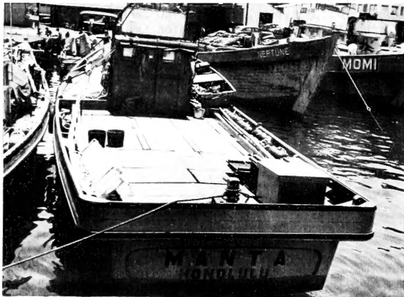
FIGURE 3 - DECK ARRANGEMENT OF A TYPICAL LONG-LINE BOAT USED IN HAWAIIAN LONG-LINE FISHING.
