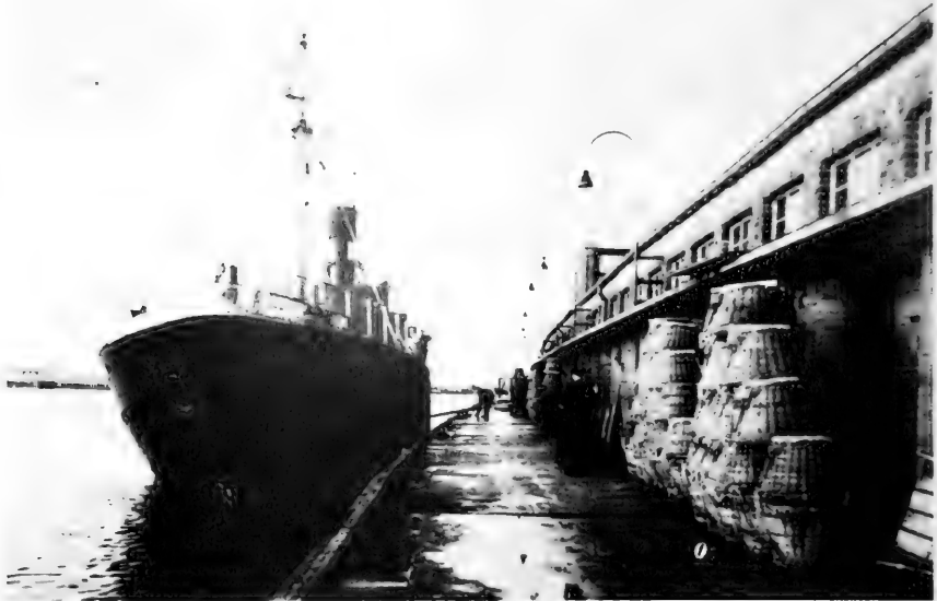
GERMAN TRAWLER ALONGSIDE AUCTION HALL X, BREMERHAVEN, GERMANY. BASKETS AT SIDE ARE USED TO DISCHARGE FISH AND HOLD ABOUT 50 KILOGRAMS OF FISH.
