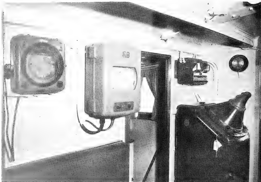
FIGURE 8 - PILOTHOUSE LOOKING AFT. NOTE THE TWO SONIC DEPTH INDICATORS, THE INTER-COMMUNICATING EQUIPMENT, SURFACE SEA TEMPERATURE RECORDER, AND THE RADAR INSTALLATION.
