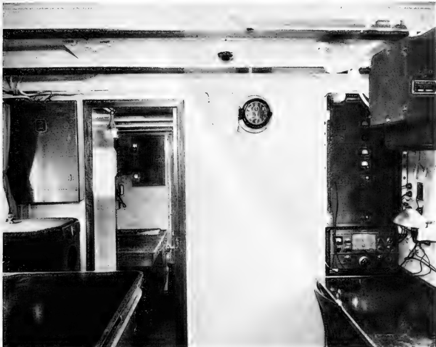
FIGURE 9 - VIEW OF CHART ROOM, SHOWING LORAN RECEIVER, 150 W. RADIO TRANSMITTER AND RECEIVER, RADAR TRANSCEIVER, AND PORTION OF LARGE CHART TABLE. THE SPACE OPENING AT THE REAR SHOWS PART OF THE ADJOINING STATEROOM.
