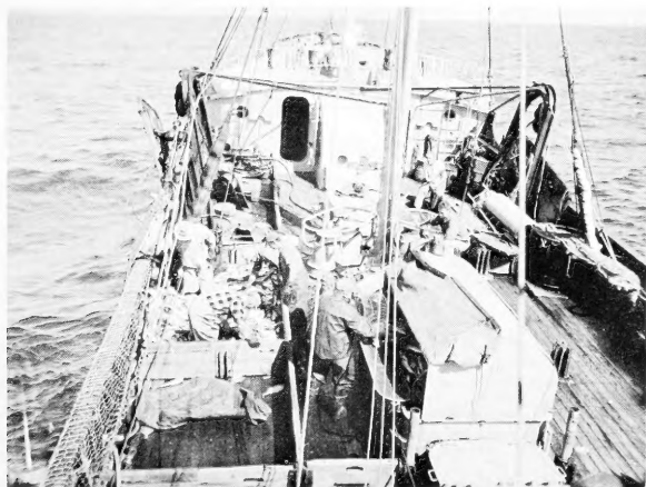
Fig. 1 - View showing location of fish charging and discharging portion of the brine-freezer tank.
