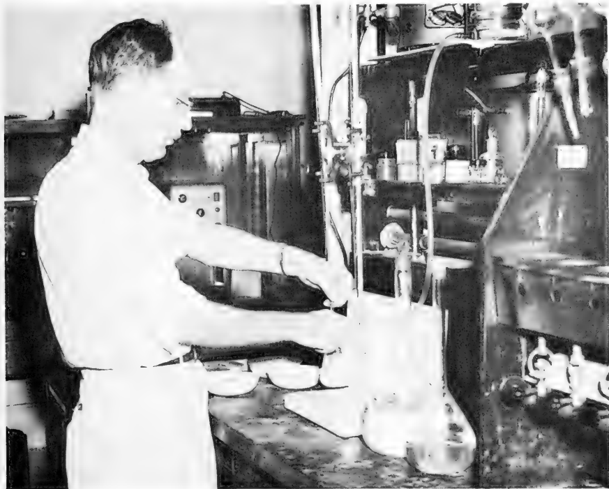
Fig. 1 - Determination of chlorides in a sample of Gulf of Mexico oysters.
