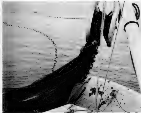
FIG. 2 - VIEW OF SARDINE STOP SEINE BEING HAULING WITH A POWER BLOCK IN THE MAINE SARDINE FISHERY.
