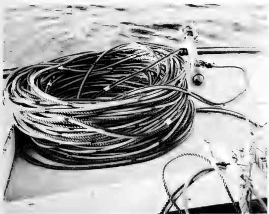
FIG. 2 - 100 FATHOMS OF PRESSURE HOSE. IN ORDER TO SUPPORT THE PRESSURE HOSE WITHOUT CONSTRICTING IT, A \frac{3}{8} " DIAMETER NYLON ROPE WAS FASTENED TO THE HOSE WITH PLASTIC ELECTRICIAN'S TAPE AT SPACES OF APPROXIMATELY 18 INCHES. THE BATHY-THERMOGRAPH WAS USED FOR CHECKING DEPTH READINGS.
