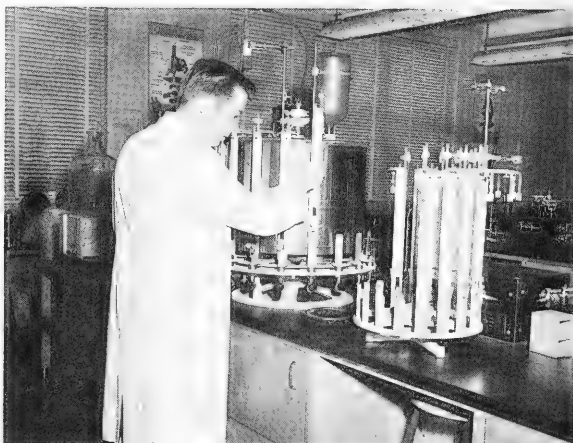
Fig. 2 - Measuring oxidation of tuna meals employing a Warburg apparatus for measurement of oxygen adsorption.
