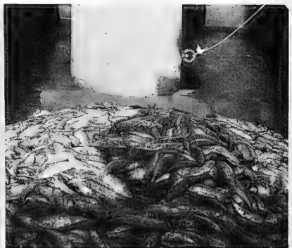
Fig. 3 - Discharge end of pneumatic fish unloader.
