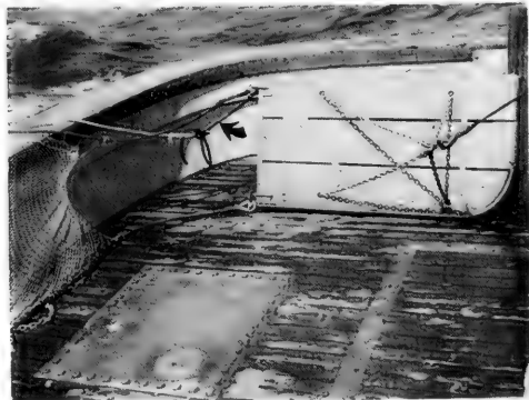
Fig. 1 - Method of attaching port door to wing of Gulf shrimp trawl. Starboard door was attached in same manner. Arrow indicates forward portion of "lazy line."
