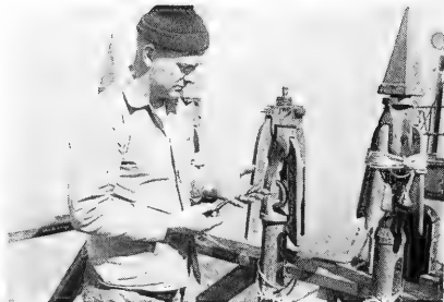
Fig. 17 - Parts of the fuse. The fuse has a plunger, which is the small part at the center of the engineer's hand. When the gun goes off, the jar knocks the plunger against a cap at the bottom of the cylinder (by the engineer's thumb of his right hand), which ignites the powder in the plunger and in the head of the fuse. This powder requires about 5 to 10 seconds to burn. It then ignites the powder in the bomb head, which explodes and kills the whale. Note the method of inserting the fuse on the harpoon in front of the engineer.
