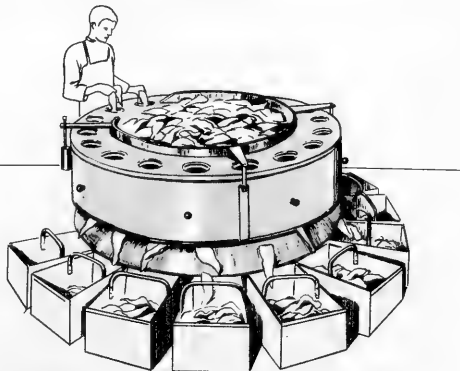
Danish fillet grading machine. Diameter--6.2 feet; height--3.6 feet.
