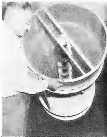
FIG. 2 - A DOWNWARD VIEW OF THE MEAL BLENDER, SHOWING THE 6-INCH DIAMETER HELICAL WORM.
