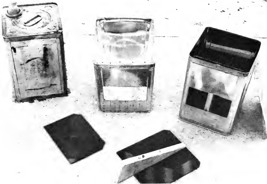
FIGURE 8.—Feed hopper (self-feeder) constructed from 5-gallon can.
