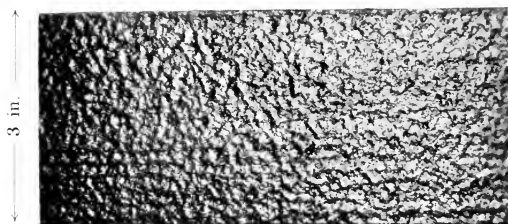
LOW MOOR WROUGHT IRON (N 20) EXPOSED TO AERIAL CORROSION AT HALIFAX FOR 10 YEARS, SHOWING POCKS AND FURROWS.
