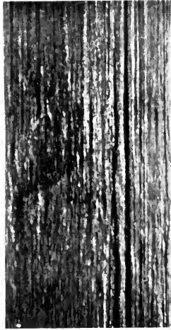
LOW MOOR WROUGHT IRON (N 42) EXPOSED (IN CONTACT WITH MILD STEEL) TO COMPLETE IMMERSION IN SEA-WATER AT AUCKLAND FOR 5 YEARS, SHOWING FURROWED STRUCTURE ON FACE.
