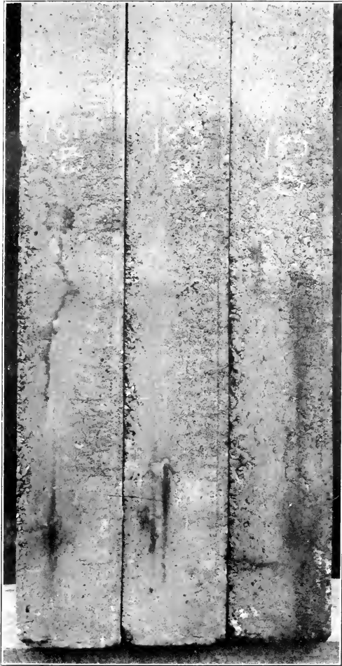
LEAN MIXTURE OF NORMAL PORTLAND CEMENT (1 : 3 : 6), NORMAL CONSISTENCY, AFTER 3\frac{1}{2} YEARS IN ARTIFICIAL SEA-WATER OF THREE TIMES NORMAL CONCENTRATION, AT WATFORD.
