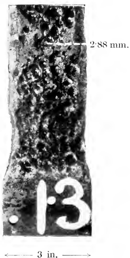
MEDIUM CARBON STEEL (E 13) EXPOSED TO HALF-TIDE CONDITIONS AT COLOMBO FOR 5 YEARS.
