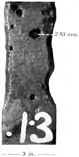
0.635 PER CENT. COPPER STEEL (G 13) EXPOSED TO HALF-TIDE CONDITIONS AT COLOMBO FOR 5 YEARS.
