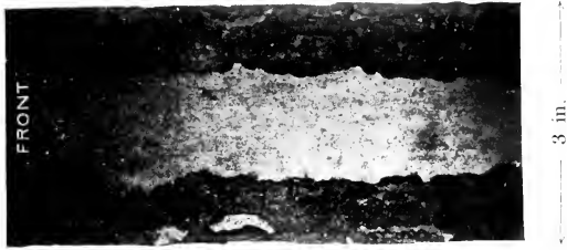
36 PER CENT. NICKEL STEEL (L 25) EXPOSED TO COMPLETE IMMERSION IN SEA-WATER AT HALIFAX FOR 5 YEARS.
