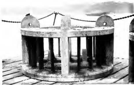
FRAME H IN SITU, CONTAINING BARS EXPOSED TO AERIAL CONDITIONS AT PLYMOUTH FOR 10 YEARS.
