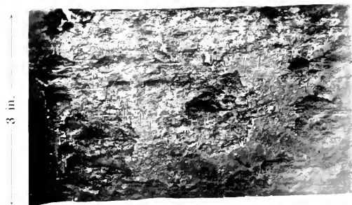
MILD STEEL (B 8), HIGH IN SULPHUR AND PHOSPHORUS, EXPOSED TO COMPLETE IMMERSION IN SEA-WATER AT AUCKLAND FOR 10 YEARS, SHOWING DEEP PITTING.
