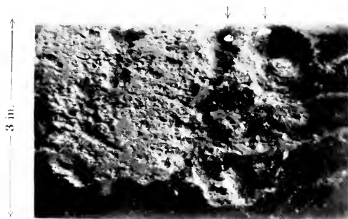
13.5 PER CENT. CHROMIUM STEEL (J 26) EXPOSED TO COMPLETE IMMERSION IN SEA-WATER AT HALIFAX FOR 10 YEARS, PERFORATED BY CORROSION.
