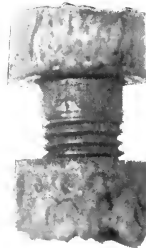
1 \frac{3}{8} in. NUT AND BOLT FROM 13·5 PER CENT. CHROMIUM STEEL (J 54) EXPOSED TO COMPLETE IMMERSION IN SEA-WATER AT PLYMOUTH FOR 5 YEARS.
