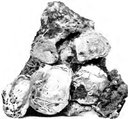
SHELLS REMOVED FROM MILD STEEL AND LOW MOOR WROUGHT IRON (C 42 AND N 42) PAIRED AND COMPLETELY IMMersed IN SEA-WATER AT AUCKLAND FOR 5 YEARS.
