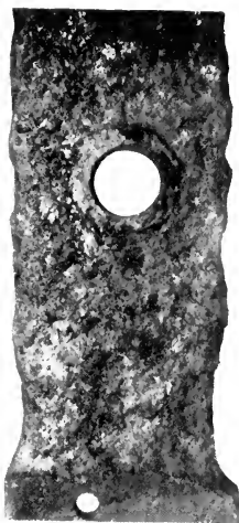
COLD-BLAST CAST IRON (R 44) CARRYING FOUR MILD STEEL BOLTS AND EXPOSED TO HALF-TIDE CONDITIONS AT COLOMBO FOR 5 YEARS.
