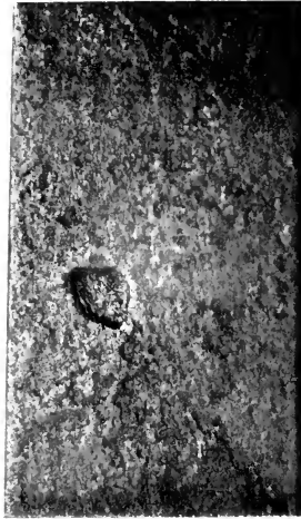
MILD STEEL (C 42) EXPOSED (IN CONTACT WITH LOW MOOR WROUGHT IRON) TO COMPLETE IMMERSION IN SEA-WATER AT AUCKLAND FOR 5 YEARS, SHOWING ISOLATED PIT ON FACE.
