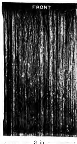
LOW MOOR WROUGHT IRON (N 69) EXPOSED TO COMPLETE IMMERSION IN SEA-WATER AT HALIFAX FOR 5 YEARS, SHOWING FIBROUS STRUCTURE.
