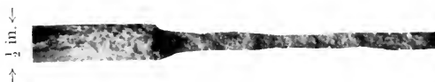
SWEDISH CHARCOAL IRON (P 2) EXPOSED TO AERIAL CORROSION AT AUCKLAND FOR 10 YEARS, SHOWING SEVERE ATTACK AT LOWER END.
