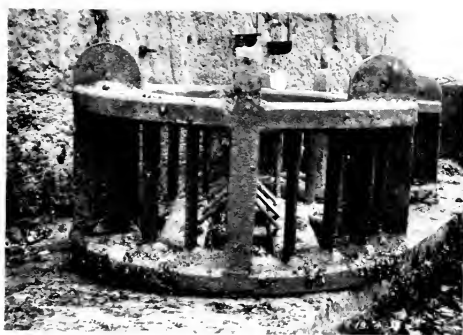
FRAME V IN SITU, CONTAINING BARS EXPOSED TO HALF-TIDE CONDITIONS AT PLYMOUTH FOR 10 YEARS.
