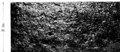
CLEANED MILD STEEL (A 26) EXPOSED TO COMPLETE IMMERSION IN SEA-WATER AT HALIFAX FOR 10 YEARS.
