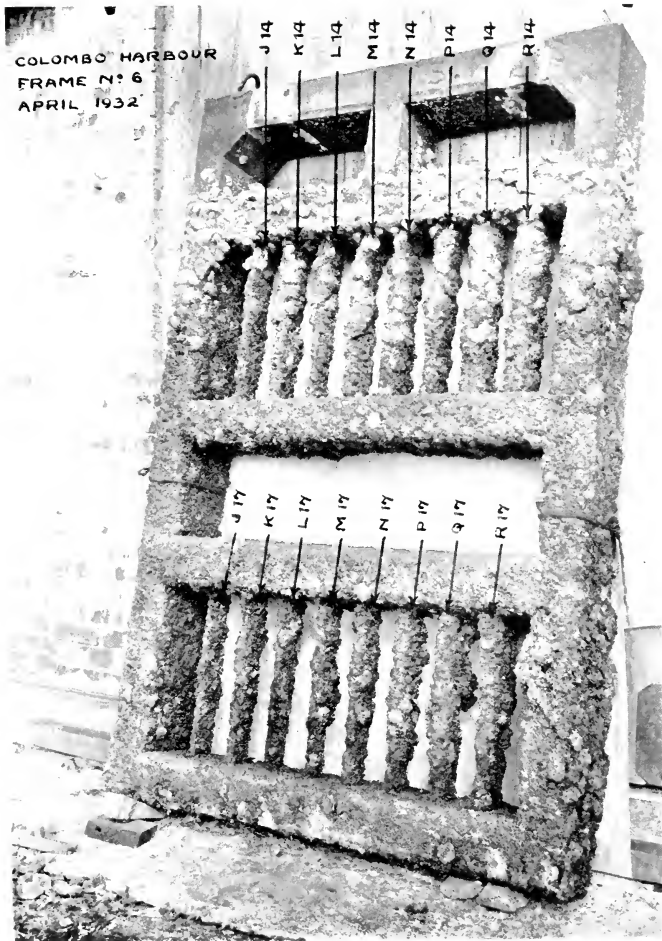
FRAME CONTAINING BARS EXPOSED TO HALF-TIDE CONDITIONS (UPPER PART) AND TO COMPLETE IMMERSION IN SEA-WATER (LOWER PART) AT COLOMBO FOR 10 YEARS.
