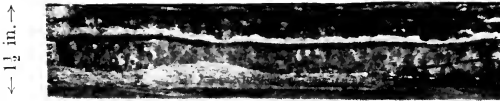
0.635 PER CENT. COPPER STEEL (G29) EXPOSED TO AERIAL CORROSION AT PLYMOUTH FOR 10 YEARS, SHOWING EDGE AND THICKNESS OF ADHERENT RUST BEFORE CLEANING.
