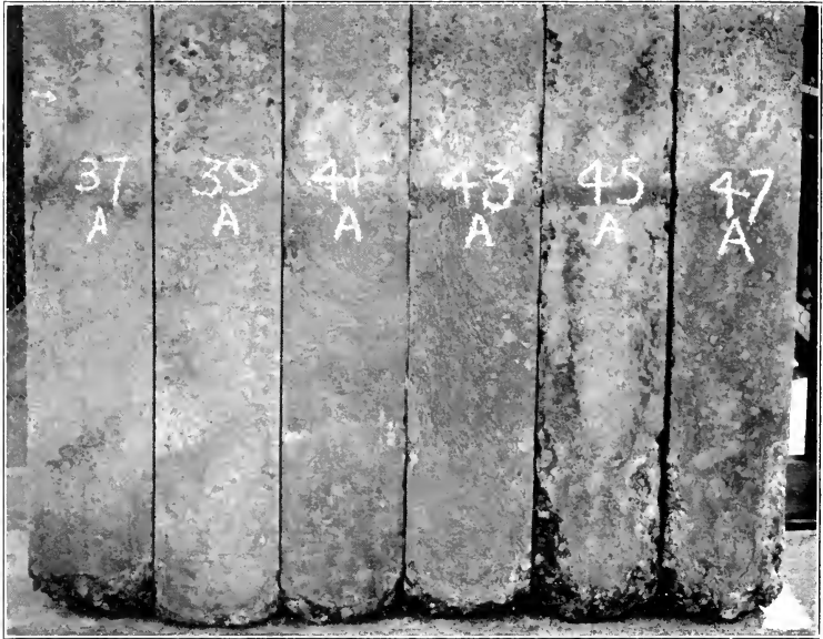
LEAN MIXTURE OF HIGH ALUMINA CEMENT (1 : 3 : 6), NORMAL CONSISTENCY, AFTER 4 YEARS IN ARTIFICIAL SEA-WATER OF THREE TIMES NORMAL CONCENTRATION, AT WATFORD.
