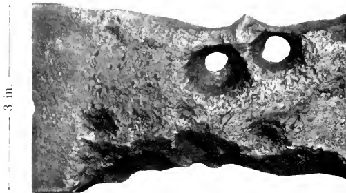
3.75 PER CENT. NICKEL STEEL (K 14) EXPOSED TO HALF-TIDE CONDITIONS AT COLOMBO FOR 10 YEARS.
