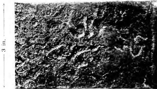
INGOT IRON (M 38) EXPOSED TO COMPLETE IMMERSION IN FRESH WATER AT PLYMOUTH FOR 10 YEARS, SHOWING VERMIFORM CORROSION.
