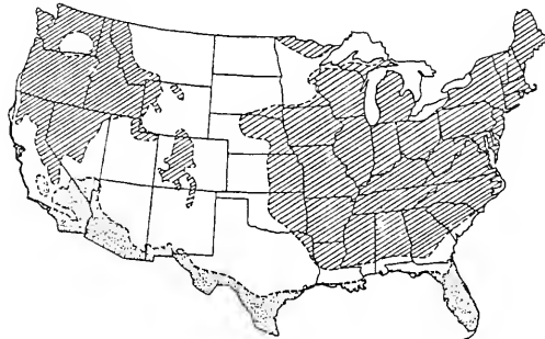
Figure 1907.1.2 Weathering Probability Map for Concrete a
