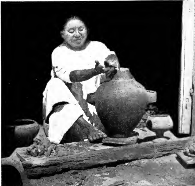
FIG. 3. — Maya woman modeling a water jar, showing the method of turning the vessel with the foot.
