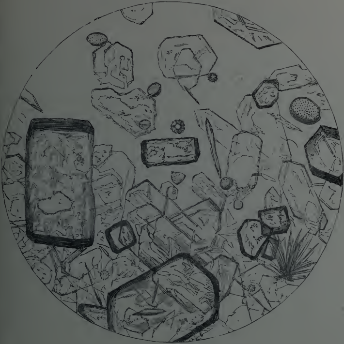
FIG. 125.—HONEY, ADULTERATED WITH CANE SUGAR: THE THICK IRREGULAR CRYSTALS ARE THE ADDED SUGAR. \times 200 .
