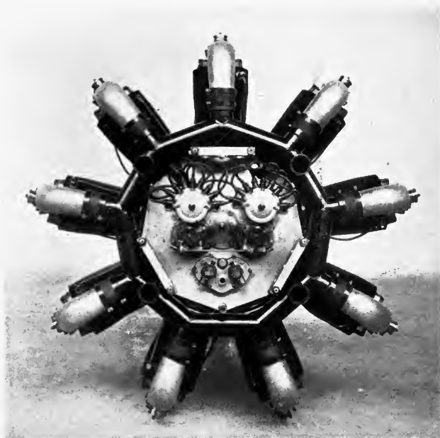
A B C DRAGONFLY 1 A RADIAL ENGINE, 340 HORSE-POWER
