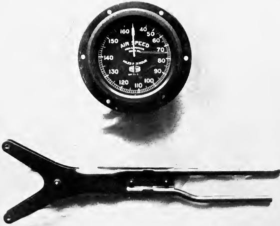
AIR SPEED INDICATOR--DIAL AND HEAD
