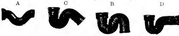
FIG. 230.—Different Forms of Traps. A , Running trap; B , S-trap; C , \frac{3}{4} S-trap; D , \frac{1}{2} S-trap.
