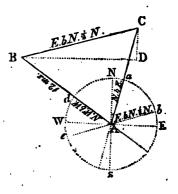
W. b. W., and E. b. S.  $\frac{1}{2}$  S., the opposite point to E. b. N.  $\frac{1}{2}$  N., is  $4\frac{1}{2}$  points = the angle ABC, measured by the arc de, and the difference between E. b. N.  $\frac{1}{2}$  N., and N. b. E., is  $5\frac{1}{2}$  points = the angle ACB, measured by the arc ab. Hence, by oblique angled trigonometry, Problem I., page 107, to find the side BC = the ship's distance from the head-land at the second station.
