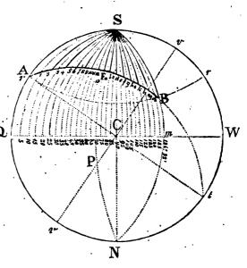
western hemisphere :---and, in the present diagram, because the ship is bound to a port to the westward of that from which she is to sail, the latter (for the sake of uniformity also) is placed on the primitive circle in the eastern hemisphere :---the letter Q representing the western hemisphere in the former case, and the eastern hemisphere in the latter.
