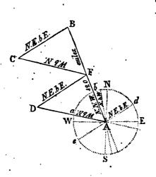
on the starboard tack, and FC, parallel to AD, the second board on that tack; let the N.E. b. E. line DF represent the first board on the larboard tack, and, parallel thereto, the line CB = the second board on this tack. And, since the ship is to make her port in four tacks, without going to the eastward of the line AB, therefore, at the end of the second tack, she must reach the point F, which bisects or divides the distance AB into two equal parts, of 60 miles each; thus making AF = to AB.
