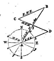
the line BC = the second board on that tack. And, since the ship is to make her port in three tacks, it is evident that the board on the starboard tack, represented by the W.N.W. line CD (parallel to dg), must bisect the line A B in the point F; and that, therefore, A F and F B are equal to one another, each being equal to 45 miles = half the line, or distance A B.
