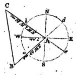
arc a b.—Hence, in the oblique angled triangle A B C, given the side A C 80 miles; the side A B 68 miles, and the included angle A = 7 points; to find the other angles, and the side B C.—Therefore, by oblique angled trigonometry, Problem III., page 179,
