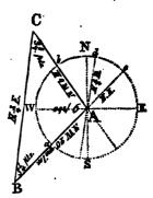
arc bd; and the difference between N.  $\frac{1}{2}$  E. and N. E. (the opposite point to S. W.) is  $3\frac{1}{2}$  points = the angle ABC, measured by the arc de.— Then, in the oblique angled triangle ABC, given the angles and the side AB, to find the sides AC and BC = the distance of the ship from the Lizard at the respective stations.—Hence, by oblique angled trigonometry, Problem I., page 177.
