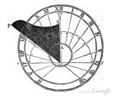
The hour lines of VII. in the evening and V. in the morning, make the same angles with the meridian, on *the opposite side of the VI. o'clock hour line*, as the hour lines of VII. in the morning and V. in the evening. In the same manner the hour lines of VIII. in the evening and IV. in the morning make the same angles with the meridian as the hour lines of VIII. in the forenoon and IV. in the afternoon; and so on.
