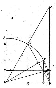
Proceeding in this manner, after 12 bisections, we come to an arc of 0°0'.52".44".3"." 45".", the cosine of which approximates so very closely to the radius C B, that they may be considered as being of equal value. Now, the absolute measure of this arc may be obtained by numerical calculation, as follows, viz.
