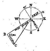
difference between S.S.E.  $\frac{3}{2}$  E. and N.E. b. E. (the opposite point to S.W. b. W.), measured by the arc *a b*, to find the angles A and C, and the true distance A C. Hence, by oblique angled trigonometry, Problem III., page 179,
