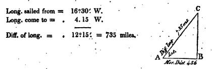
Solution.—In the right angled triangle ABC, let the hypothenuse AC represent the difference of longitude; the angle A, the latitude of the parallel; and the base AB, the meridional distance: then, there are given, the side AC = 735 miles, and the leg AB = 456 miles, to find the angle A. Hence, by right angled plane trigonometry, Problem III., page 174,
