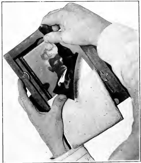
Illustration No. 2 Removing Dust from Neg- ative while Printing See Paragraph No. 43
