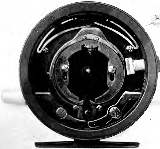
FIG. A.—PLAN SHOWING INTERIOR MECHANISM OF THE FRED G. SHAW SPINNING REEL. THE TWO PAWLS, SLIDING PLATE, SPRINGS, THE LEVERS AND THEIR HANDLES AND THE BUTTERFLY NUT.
