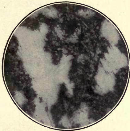
FIG. 119. — Martensite, black. Troostite, white. Magnified 350 diameters.
