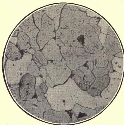
FIG. 111. — Ferrite with very thin continuous cementite skeleton. Low carbon. Magnified 250 diameters.
