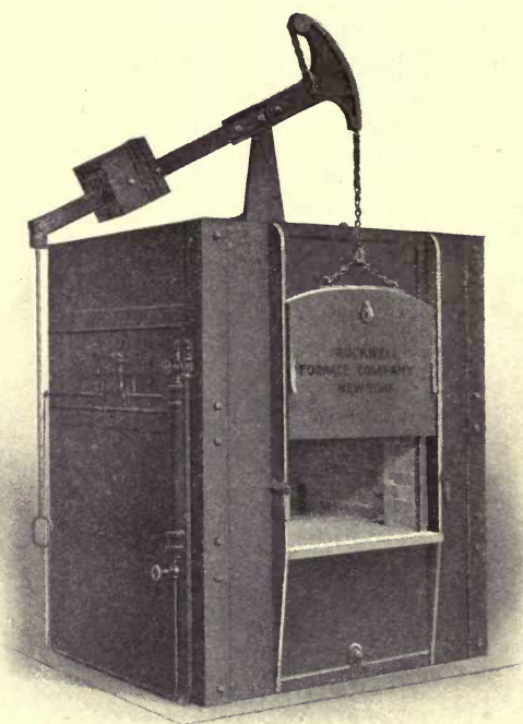
FIG. 81. — Small over-fired furnace.
