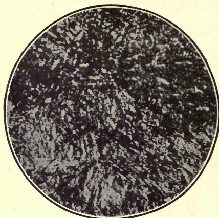
FIG. 115. — Martensite formation. Magnified 250 diameters.
