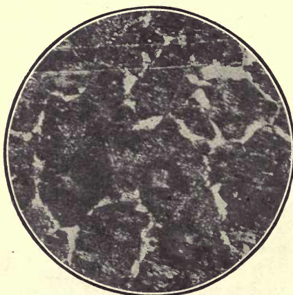
FIG. 113. — Ferrite matrix with separated pearlite islands. Magnified 250 diameters.
