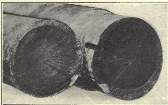
Fig. 60. — Piece forged with relatively light hammer.
