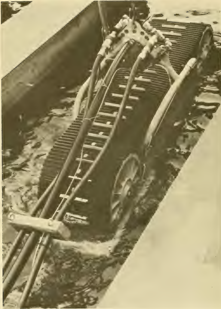
Figure 41. Test track described in Nuttall (1970a) in water at Chesapeake Bay, supported between the pontoons of WNRE's test rig.
