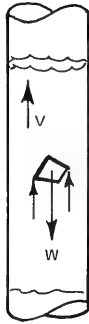
Figure 53. Forces acting on a dense, falling particle in a vertically moving stream of fluid.
