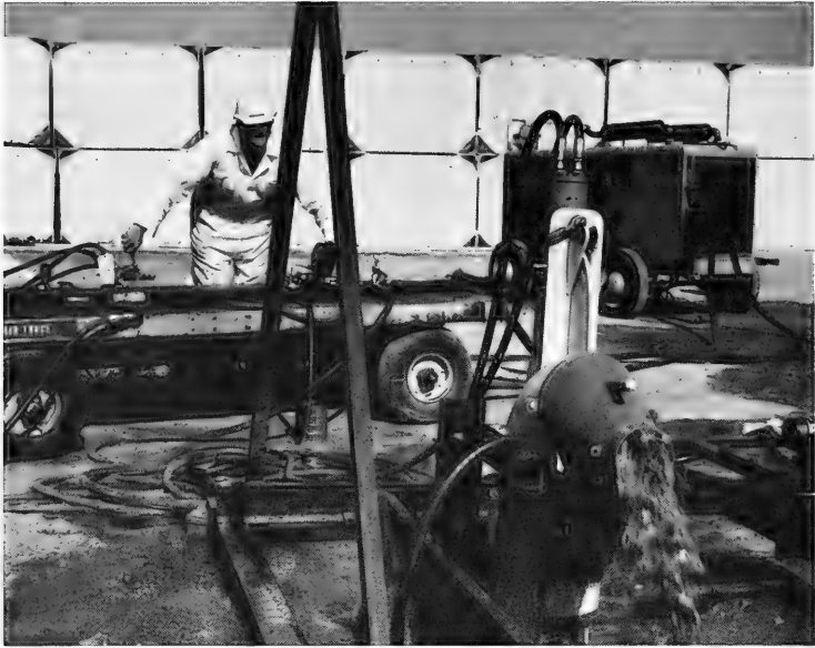
Figure 55. Soil cutter and pump undergoing preliminary testing at NCEL, working in a hole filled with water in hard, rocky soil.
