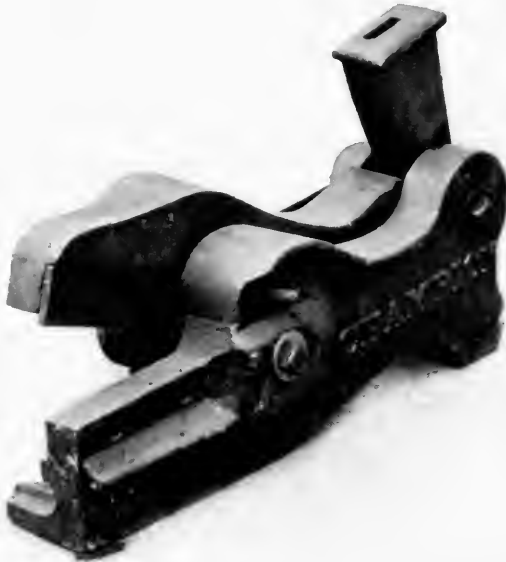
Fig. 75.—Hand shear for cutting reinforcement.
