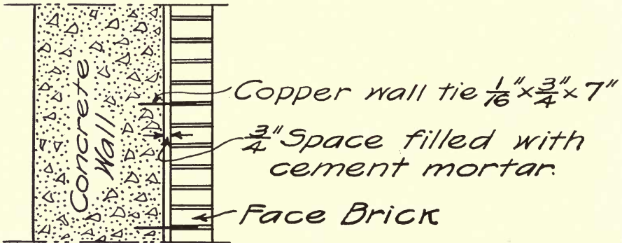
Fig. 19.—Brick Wall Ties. (See p. 68.)
