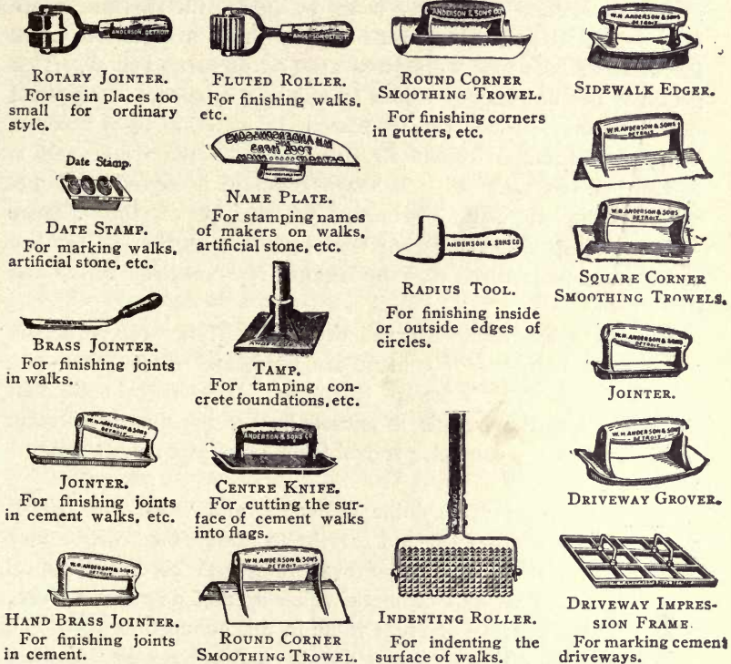
Fig. 60.—Tools Used in Finishing Cement Surfaces.
